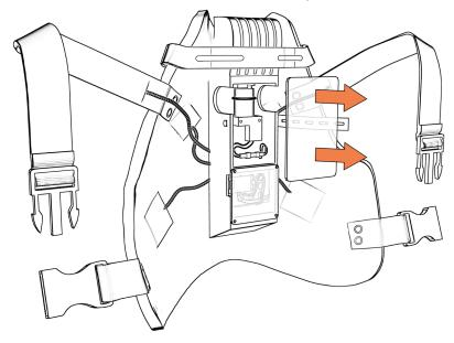
**2** Disconnect electrical connection of mucus chamber.
