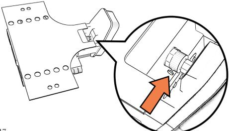
**d.** While holding down the metal switch with one hand, use the other hand to pull the genitalia straight back until it is completely off the guide rail system.
