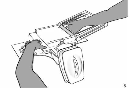
**C.** Insert urine bag under the white roller and attach to side of the device with thumb screw.
