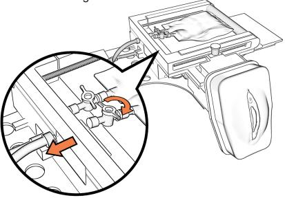
**3** Remove urine bag – be careful opening and closing the bladder mechanism.
