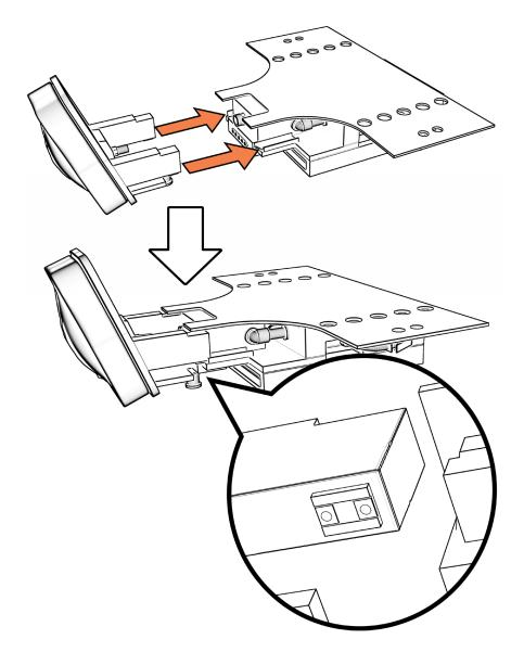
**d.** Slide the carriages in all the way down the guide rails until the metal fitting on the genitalia meets the metal housing on the yellow compartment
