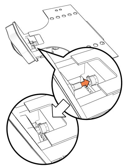
**f.** Turn the device back over. Gently lift slightly up on the spring plunger and twist slightly to the right to let the head to all the way down. The genitalia should be locked and sturdy.
