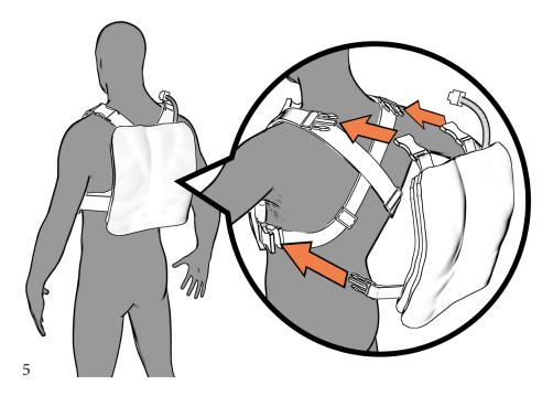
**5** Connect the electrical connection from the chestplate to the backplate.
