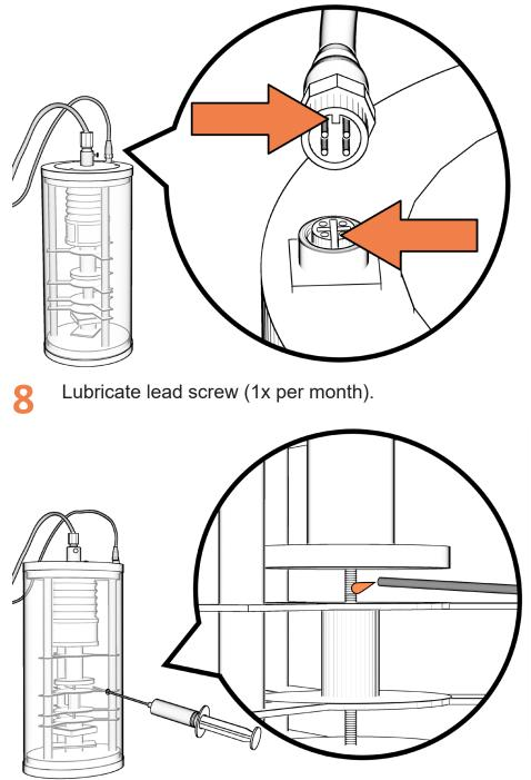
Plug power cord into bottom of device.
