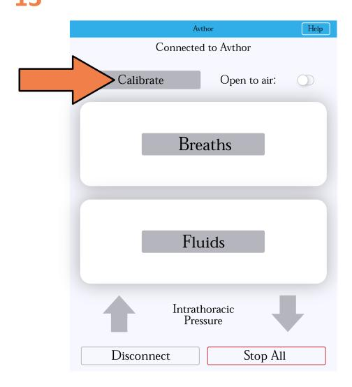
14 On the app you can set the breath rate, blood flow rate, intrathoracic pressure, and create an air leak with the open to air button.
