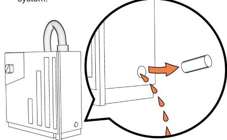
9 Flush drainage system through hole with distilled water and use small tube and syringe to suck excess water out of system.
