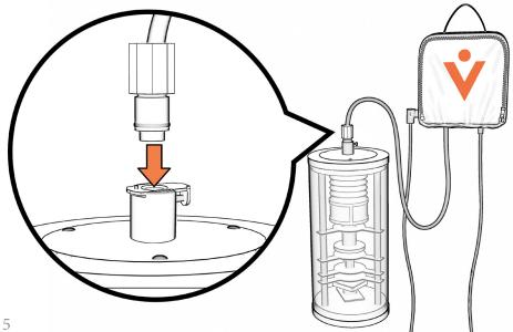
(you might need to compress the floor unit connector to allow the connectors to go together)
