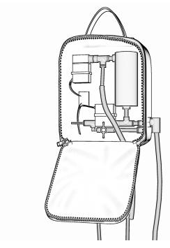
Open the valve at the bottom of the back pocket.
