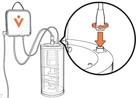
(Line up the notches for the two electrical connections)
