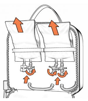
Disconnect tubing from ribs and flush ribs with distilled water.
