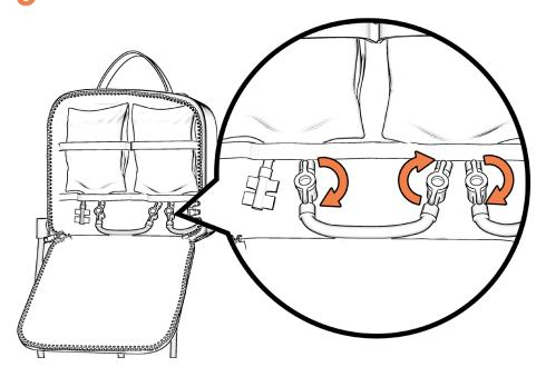
Connect electrical connection from control bag to floor unit.
