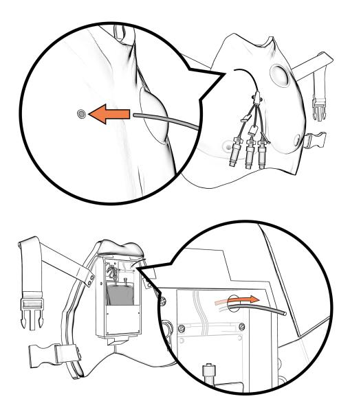
Install connector on central line inside chest plate.
