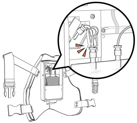
2 Remove port-a-cath- from device by sliding out port-a-cath housing.
