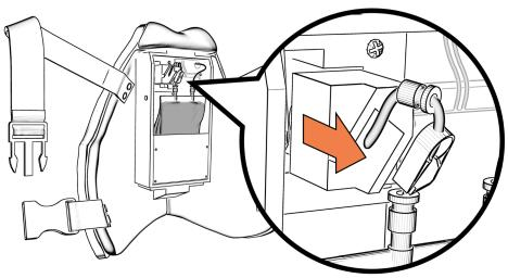
Remove port-a-cath from device by sliding out port-a-cath housing and disconnecting tubing connection.
