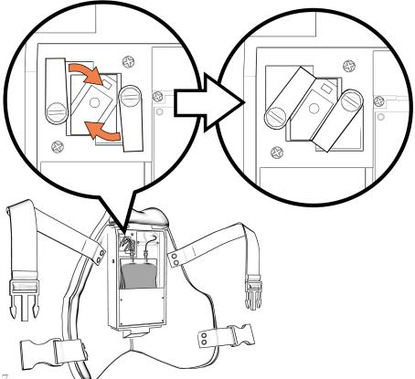
Attach electrical connection to Port-a-cath housing.
