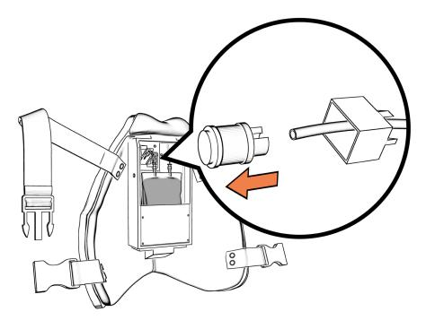
4 Pull out silicone insert from port-a-cath and wipe down both the plastic and silicone components with paper towel. Snap the silicone back into place when complete.
