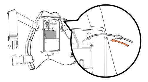
Remove red cap from central line side of blood bag. Thread central line into blood bag until there is a little slack outside of the bag. Screw on cap that is on central line to blood bag.
